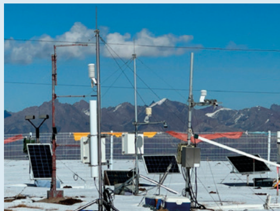
Example of an INARCH automated hydrometeorological station deployed to a high mountain basin: Qilian Mountains, China
