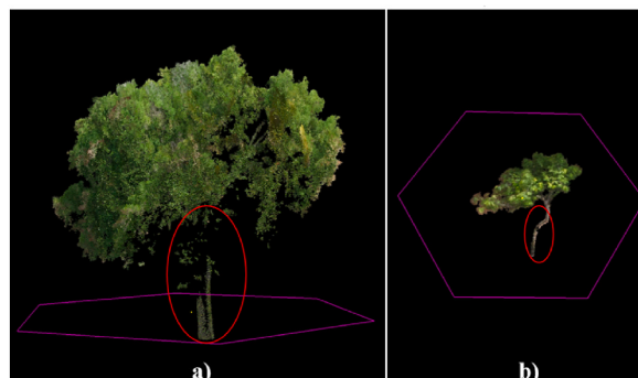
Fig. 13. Comparison of Canopy Density Effects on LiDAR Point Capture of the Trunk: (a) Dense canopy limiting point capture on the trunk; (b) Lower canopy density enabling greater definition and trunk registration.
